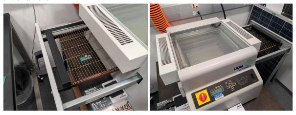
To start the reflow, press both side buttons simultaneously.
