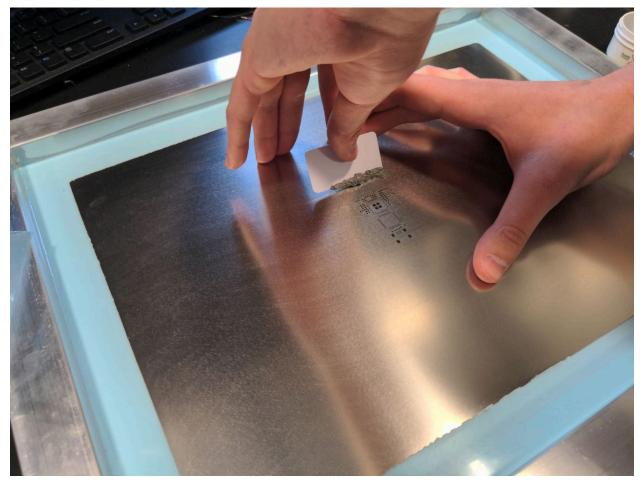
Make sure the stencil aligns with the pads on your board. You may want to tape the board to the stencil to keep it from moving around.
