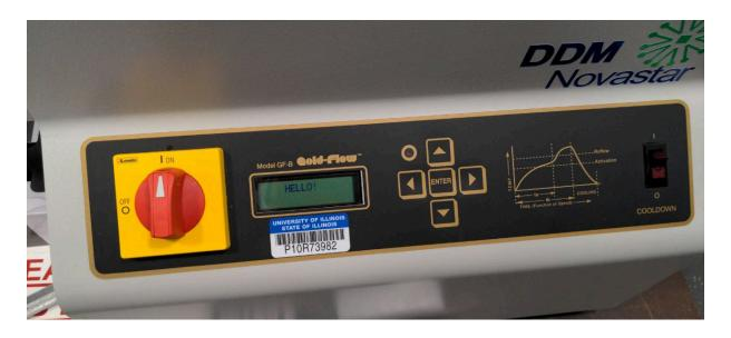
If the oven is not on and preheated, turn on the oven by turning the red knob to the "ON" position. Navigate to the "PROFILE" menu. And confirm the temperature,  $t_a$  and  $t_b$  are correct. Consult the datasheet for your soldering paste for exact values. The temperature at the top of the screen should be the peak temperature of the paste.
