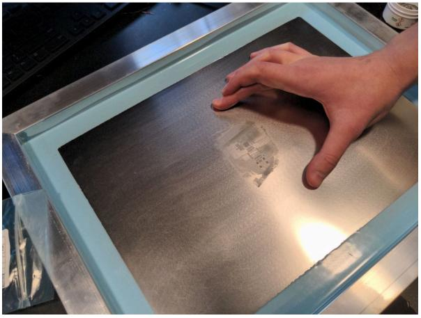
You can use a squeegee or old credit card as a spreader. You can find paste in tubs in the red mini-fridge under the soldering oven.
